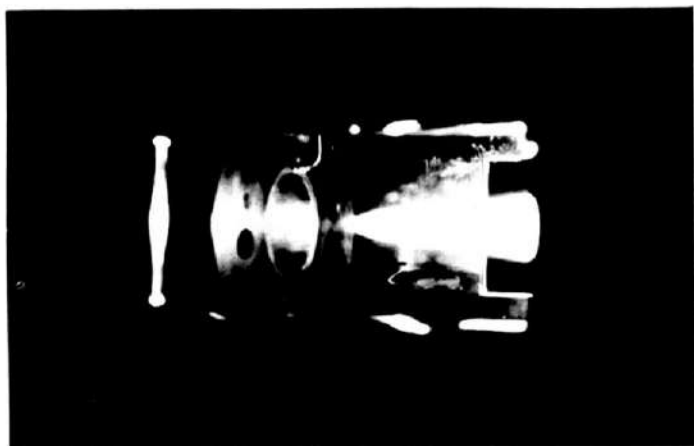
Fig. 30. Direct photograph of air-hydrogen combustion; T_{s_e} = 1300^\circ\text{K} ; T_{s_j} = 970^\circ\text{K} ; u_j/u_e = 0.28 .
